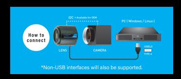
I2C interface can be used with LensConnect-compatible cameras.
