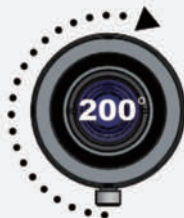
Existing Lens Focus ring rotation angle: 200°
