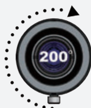
Existing Lens Focus ring rotation angle: 200°
