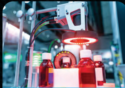
Remote compensation of focus shift for each wavelength in inspections using multiple wavelengths
